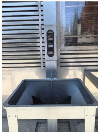
vertical bucket elevator
